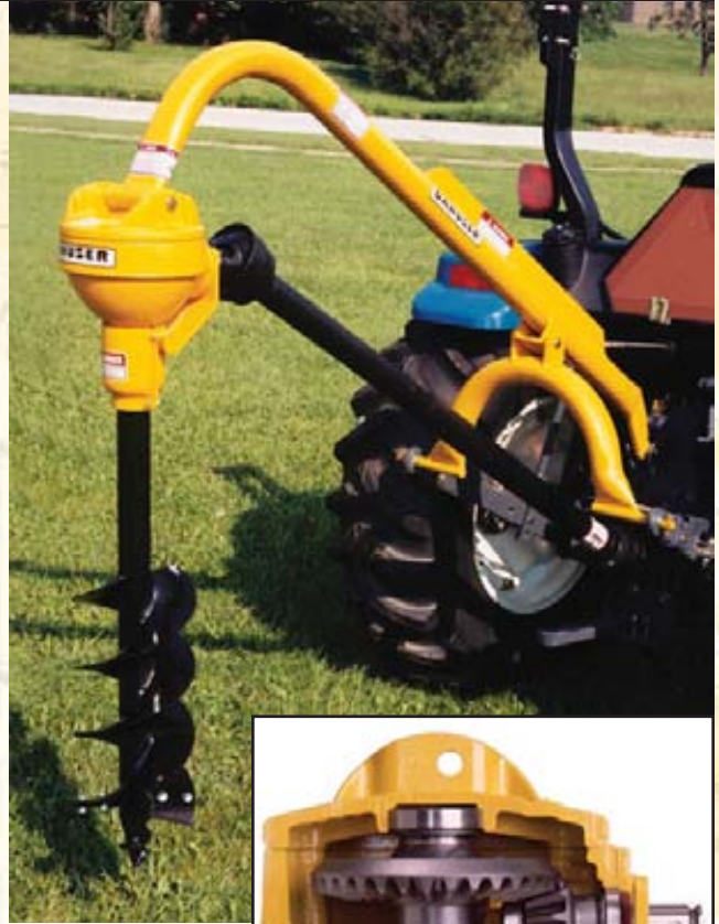
G20/40 & J20/80 gearbox cut-away with one quarter of Auger Adapter Guard removed
